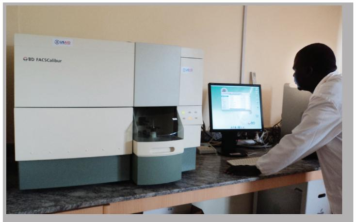
*After:* A laboratory technician at Fort Portal RRH conducts CD4 count analysis using the newly-procured FACS Calibur machine installed in the renovated space.
